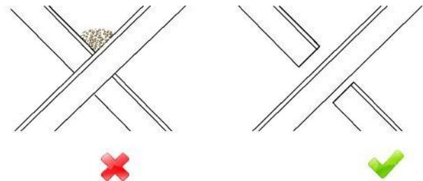
Figure 3c - Prevent water and dirt from remaining behind on joints by means of breaks
